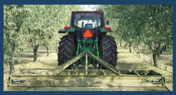
The concept is straightforward. Initially, the ORCHD Leveler cuts through and gathers soil towards the center, followed by pushing the soil back outward, consistently cutting and filling. The rear smoothing plate or roller serves as a stabilizer, firming and flattening the ground. The curved reversible cutting blades effectively slice through soil, debris, and vegetation, functioning similarly to a road grader blade. The blade mounts have slots, allowing for adjustments to the cutting depth.
